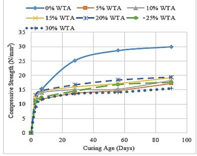
Figure 4: Compressive Strength of WTA- Mortar
