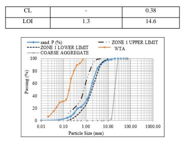
Figure -1: Particle size distribution of WTA, fine & coarse aggregates
