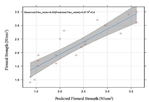
Figure 3: Predicted Versus Observed Values for Flexural Strength of WTA - Mortar
