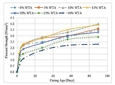
Figure -2: Flexural Strength Development of WTA – Mortar
