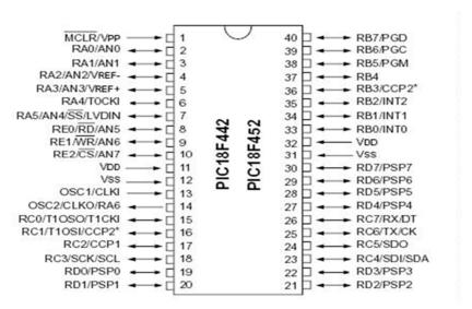
Figure 6: PIC18F452 microcontroller Pin Configuration
