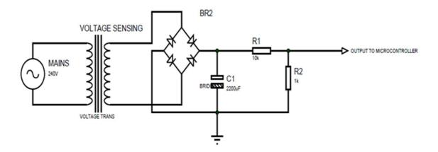
Figure 4: Voltage sensing circuit
