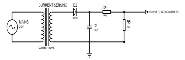
Figure 5: Current sensing circuit
