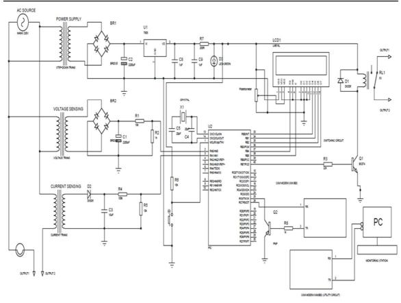
Figure 3: Complete Schematic diagram for AEMS\_GSM
