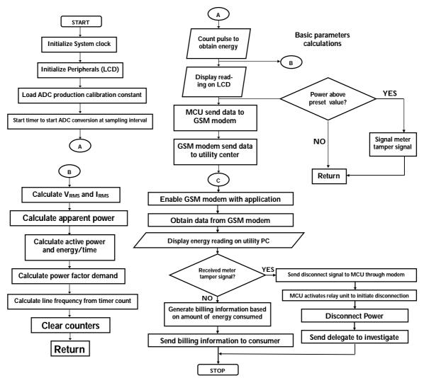
Figure 7: Flow diagram for the Automatic Metering System (AEMS\_GSM)
