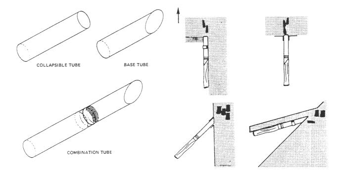
Figure 3. Constantine's bat excluding device includes a rigid base tube which attaches to the roost opening and a pliable, collapsible tube attached to the distal end. The excluder can be attached in different configurations for different situations. (Reproduced from Greenhall 1982).
