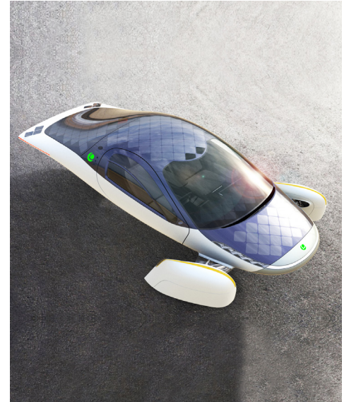
Above: Diamond-shaped solar panels on the Aptera. Photo/Aptera.
