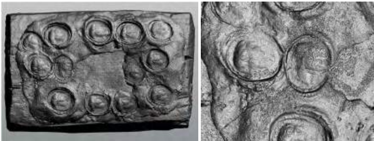
Fig. 15 and Fig. 16. Front view in solid mode of the photogrammetric model (left). Detail of the surface in solid mode of the same model (right). The distortion of the surface by a soft noise is evident. Although the general shape has been correctly captured, the fine details that could be enhanced with RTI with photogrammetry cannot be visualized. Authors.
