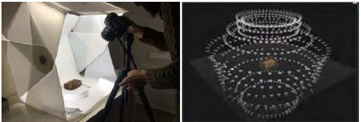
Fig. 5. Image during the photo capture process with a semi-automated shooting thanks to the synchronization of the turntable with the camera (left). Fig. 6. Image of the photogrammetric model creation process with the RealityCapture® software (right). Authors.
