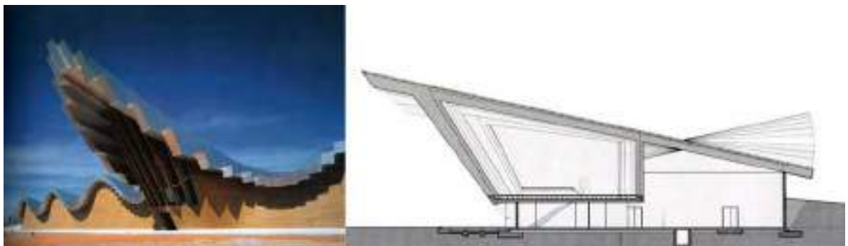
Fig. 3. In the example, the photograph is a section of Santiago Calatrava's Ysios Winery. The image shows how the section contains only the geometric information of a small portion of the real model that changes in space, published in Jodidio (2005).
