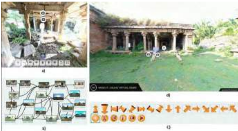
Fig. 5. Interface of the online VT builder (a) Hotspot editor, (b) Transition map, (c) Available icons for navigation and embedding ancillary data (d) Final output.
