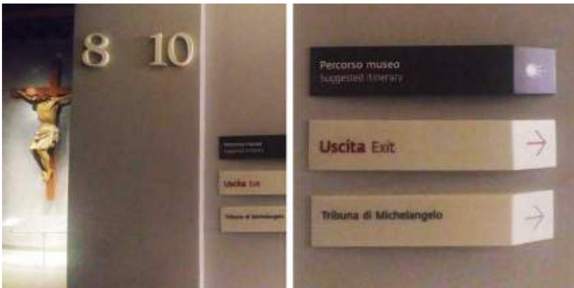
Fig. 2. Museo dell'Opera del Duomo, Florence (Italy). Design by Natalini Architetti, Guicciardini e Magni Architetti. Example of misleading information: the numbering of the rooms does not follow a logical order. The graphic design of the suggested itinerary seems to indicate going back.
