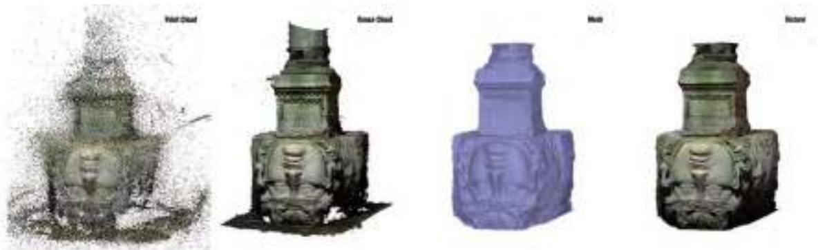
Fig. 3. Photogrammetric process phases by Agisoft Metashape (Photoscan) – Medusa's Head sculpture.
