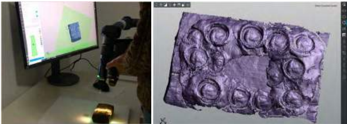
Fig. 7. Image during the 3D scanning process with the laser scan arm. Fig. 8. Image of the software process for data acquisition. Authors.
