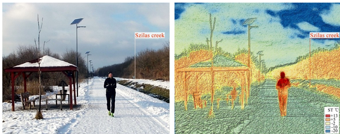
Fig. 12 Surface temperature (ST) differences in a patchy snow-covered side Szilas creek (XVI. District) (taken at 13:59 on 12.01. 2019).
