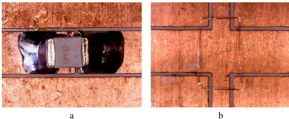
Fig. 2.42: a) SMD capacitor mounted on the series gap. b) Air bond-wires connecting the ground planes at the base of the stub to the central CPW line
