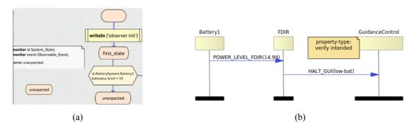
Figure 2. Examples of properties with TASTE: (a) Boolean stop condition / dynamic observer modelling an error if the battery level is lower than 10 units, (b) MSC property modelling that if the battery level drops below 15 the FDIR stops the system.
