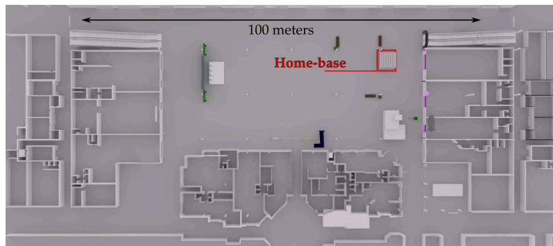
Figure 8.4: The 3D mesh model of the real mall in Finland. The entire mall having a size of 528.6 meters per 247.5 meters on two levels, we have only modelled the part which can be visible from the interaction area. It results in a model of 150 meters per 69 meters.
