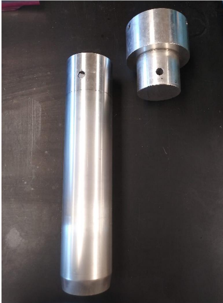
Figure 5. A stainless steel sleeve was fabricated to protect the transparent mylar cylinders from buckling during soil sampling on golf course putting greens.
