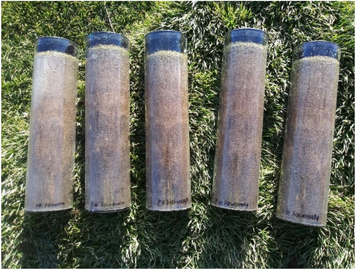
Figure 6. Soil cores 30 cm in length taken from the practice putting green at Mahoney golf course in Lincoln, Nebraska. Soil cores were taken in transparent cylinders in order to capture flow patterns with time lapse photography during the dye tracing experiment.
