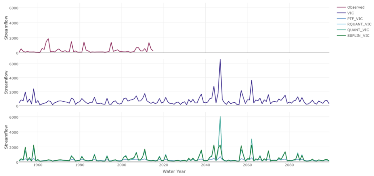
Figure 7.18. USGS Gage Spearfish Creek at Spearfish, SD; examples of downscaled GCM (BCC-csm101_rcp85_r1i1p1). The figure shows the hindcast and scenario for future annual maxima plots for the VIC hydrological model. Quantile step size is 0.01%.
