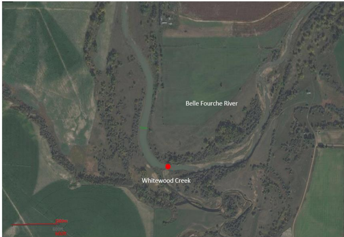
Figure 1.14. Google Earth imagery from Oct. 1, 2016. The red point indicates the confluence of Whitewood Creek and Belle Fourche River at 44.6402N latitude-103.4614W longitude. Channel width on the Belle Fourche River is represented by the green line upstream from its confluence with Whitewood Creek. Channel width at that point is approximately 100 feet. Notice that the channel characteristics change, indicating a more braided channel consistent with an increase in sediment load. Stream width decreases by about half, to approximately 50 feet.
