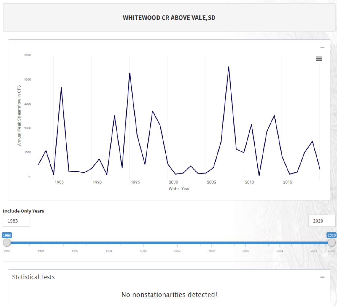
Figure 7.7.1. USGS Gage 06436198-Whitewood Creek Above Vale, SD plot of non-stationarities identified for Instantaneous Peak Streamflow (IPS) using annual peak streamflow in cfs, for years 1983-2020. The Bayesian Change-point Test was not applied as the assumption of normality was not met. No non-stationarities were detected.
