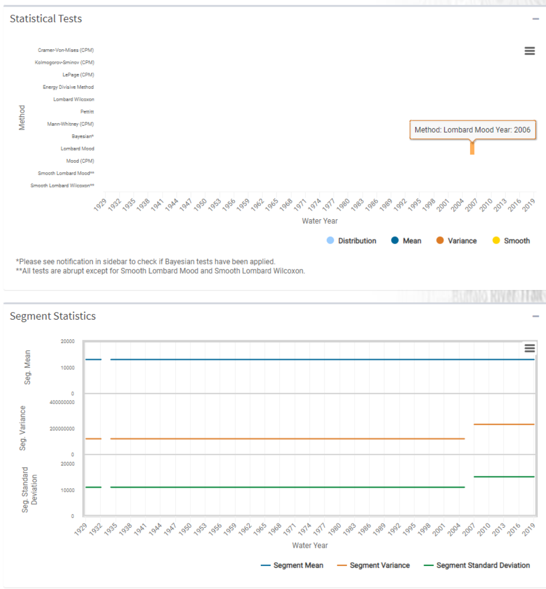
Figure 7.9.2. USGS Gage 06438000, Belle Fourche River Near Elm Springs, SD, plot of non-stationarity identified with the NSD tool identified for Instantaneous Peak Streamflow (IPS) using annual peak streamflow in cfs, for years 1929-2019 using NSD tool version 2.0.: Variance, Lombard Mood in 2006.
