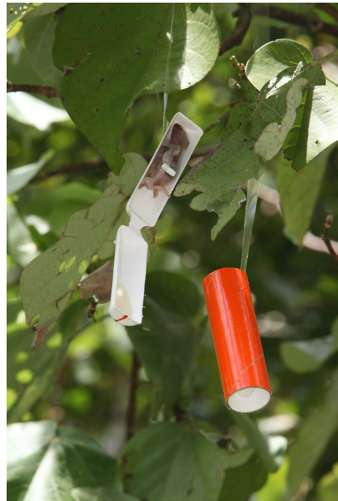
Figure 1. Deployed bait cartridge suspended within canopy vegetation. The bait mouse and acetaminophen tablet are lightly glued into the capsule and exposed for consumption by arboreally foraging brown treesnakes on Andersen Air Force Base, Guam, USA, 7, 10, and 14 June 2019. All cartridge components are biodegradable. Photo is by S. R. Siers.
