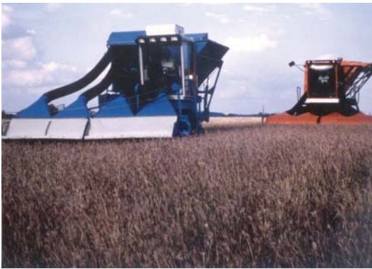
FIG. 32.7. Stripper harvesters are designed to make multiple harvests from the same native grass stand in the same year. These machines come in widths from 1 to 8 m to fit different kinds of terrain. They can be powered by hydraulic motors, combustion engines, or tractor power take-off systems and can be mounted on a combine, tractors, jeeps, and all-terrain vehicles, as well as hand-held units. This technology greatly increases the ease of harvest of chaffy native seeds.
