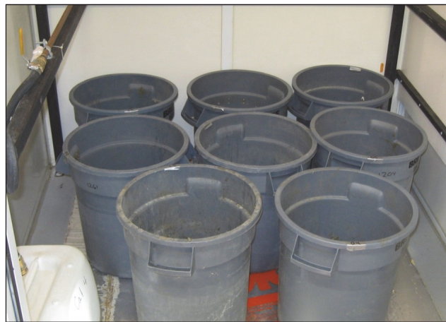
Figure 1. Lab-scale bedded packs containing bean stover, corn stover, pine wood chips, and wheat straw in environmental chambers.
