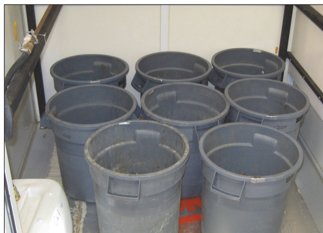
Figure 1. Lab-scale bedded packs containing corn stover, bean stover, wheat straw, or pine wood chips and stored at cool (15°C) or hot (30°C) temperatures in environmental chambers.
