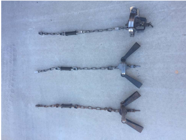
Figure 1. Three models of foothold traps: number 11 double long-spring trap with double jaws (bottom), number 11 double long-spring trap with standard jaws (center), and number 2 coil-spring trap (top) used to capture 70 river otters Lontra canadensis to assess trap-related injuries in Arkansas, Missouri, North Carolina, and South Carolina during 1999 to 2007. Chaining systems were consistent among trap types. All three trap types met animal welfare criteria established within the Best Management Practices for Trapping program.
