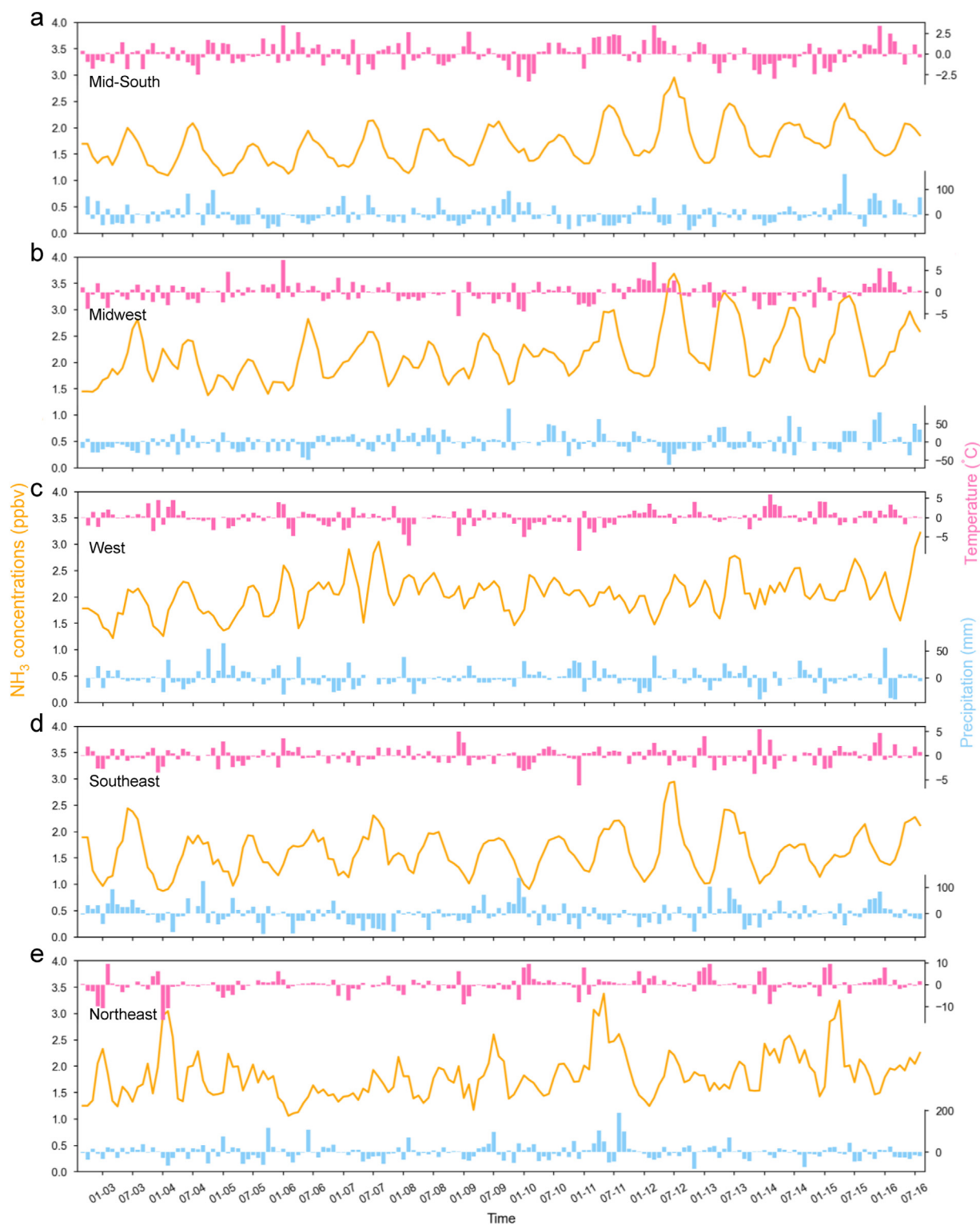
Fig. 3. Temporal changes in monthly \text{NH}_3 concentrations, temperature anomalies, and precipitation anomalies in the five US regions from 2002 to 2016. Monthly \text{NH}_3 concentrations are shown as 5-month moving averages. Monthly temperature and precipitation anomalies were calculated by subtracting the 14-year average of each month.
