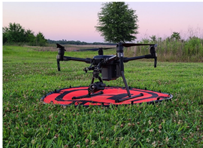
Figure 1. Small, unmanned aircraft system used in this study—Quadcopter—DJI Matrice 200 V2—equipped with visible/thermal sensor payload—Zemuse XT2—that was used to capture imagery.
