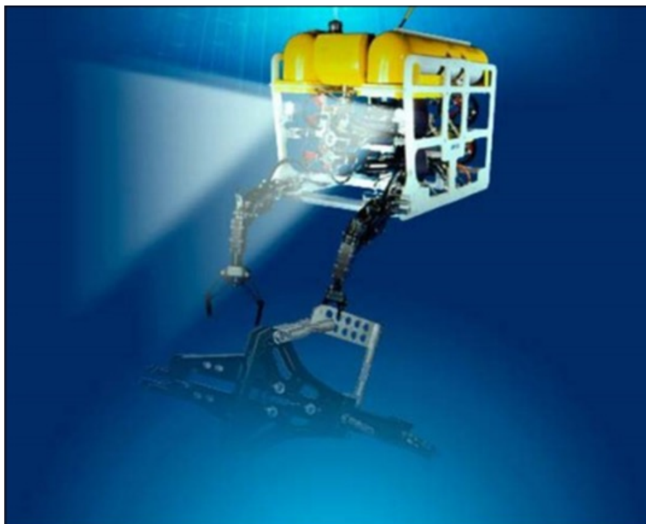
FIGURE 7: REMOTELY OPERATED VEHICLE (ROV) IXV
