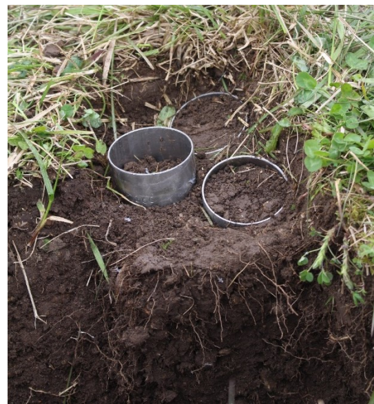
Figure 5: Soil cylinders in an A-horizon (own photo 2021)
