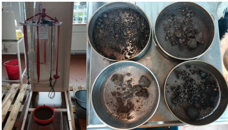
Figure 6: Cornell Sprinkle Infiltrometer (left) and stable aggregates after rain simulation (right) (own photos 2021)
