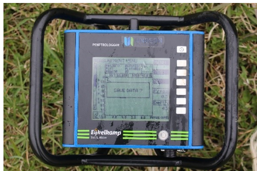
Figure 7: Penetrologger used in the field (own photo 2021)
