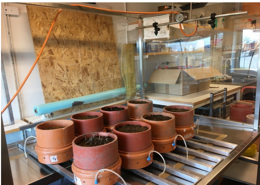
Figure 8: Eight lysimeter samples placed in rain simulator at the Soil and Environment department at SLU (Own photo 2021).
