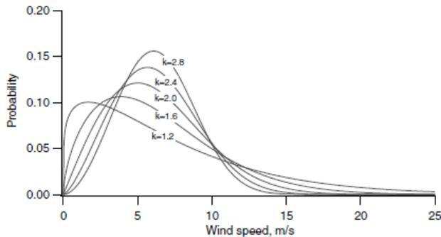
Figure 2: Weibull probability density function for  $\bar{U} = 6$  m/s [2]
