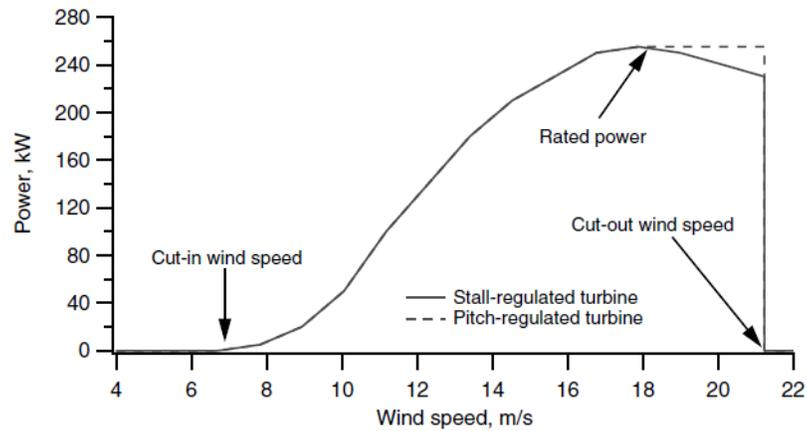
**Figure 1: Wind turbine power curve [2]**
