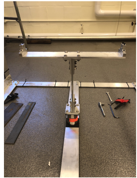
(b) Tee, center beam, and load cell interface
