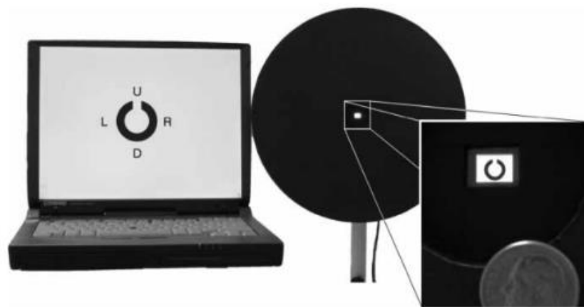
Figure 2.18 - Landolt-C optotype as projected on a laptop screen (used for the “far” target at a distance of 4.0 meters) and a microdisplay (used for the “near” target at a distance of 0.5 meters) - Figure taken from Peters and Bloomberg (2005).
