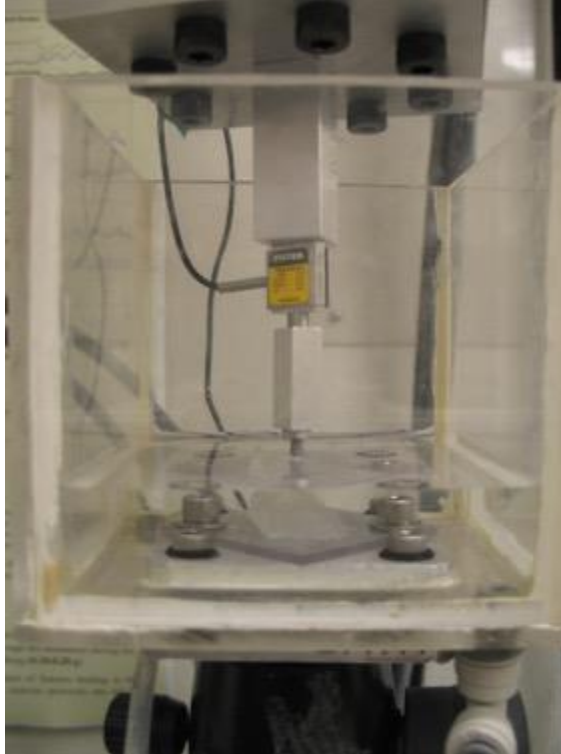
Figure 2. Upper Set Up for Indentation Testing (note this image was during testing and thus includes the wedge mount with specimen attached)
