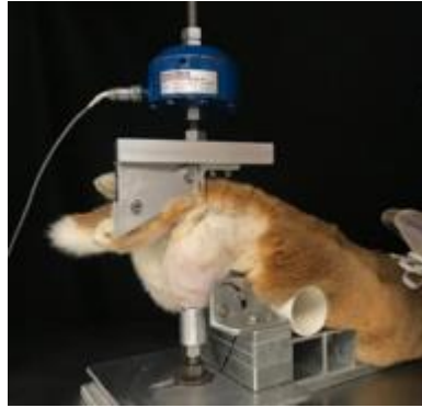
Figure 13. Injurious impact of rabbit knee set-up. In prone position (belly down) the rabbit's hind paw is supported directly below the actuator of an Instron and the knee is supported to prevent lateral and medial motion.
