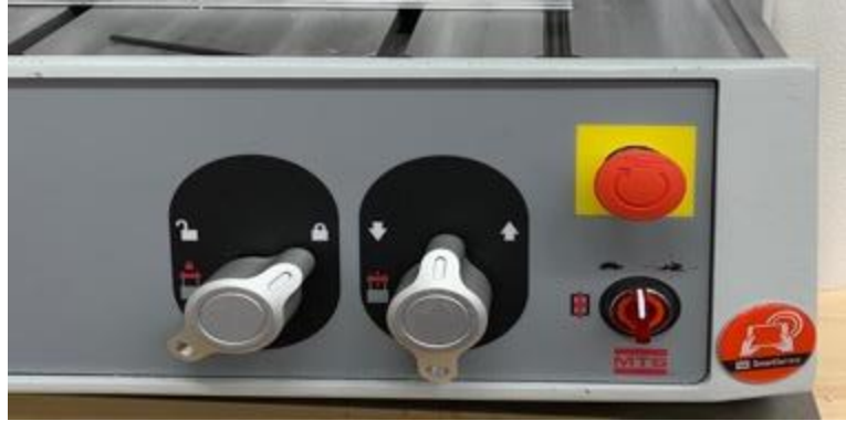
Figure 2. Front switches of MTS. Left switch locks and unlocks crosshead. Middle switch moves crosshead up and down, when unlocked. Bottom right switch indicates turtle or rabbit mode. Large red button is emergency stop button.
