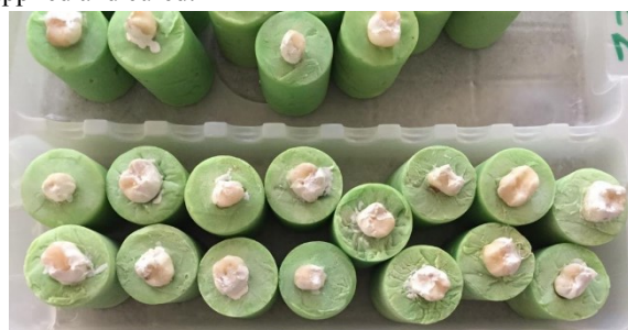
Figure 1- Mounted samples in self-cure acrylic resin
