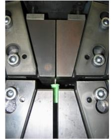
Figure 3- Load application to determine the force required for post retrieval from the root canal system
