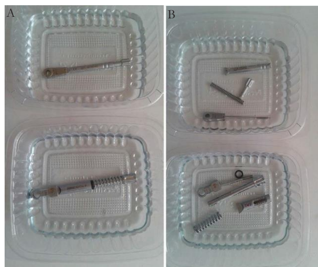
Fig 2. Assembled (A) and dismantled (B) form of FS-MTLDs. Top: Astra Tech. Bottom: Dr. Idhe.
