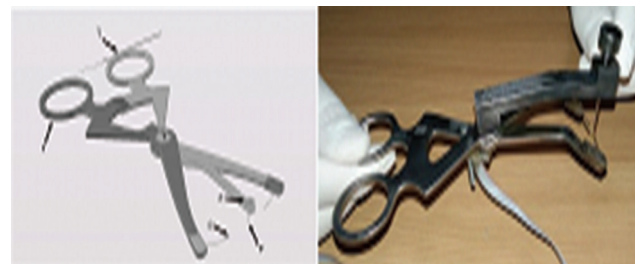
Fig 3. Mechanical part of the gauge includes (I) handles adjusting the horizontal pins, (II) location of magnet and IC magnetic sensor, (III) vertical pin, (IV) horizontal pin, (V) screw to adjust the vertical pin and (VI) wire connecting the magnetic sensor to the main circuit.
