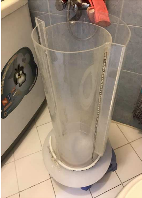
Figure 2. A calibrated container was used to Water displacement volumetry
