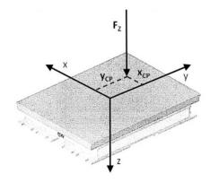
Figure 2. Determine the Center of Pressure Using Measured Forces and Moments.  $^{\rm 13}$
