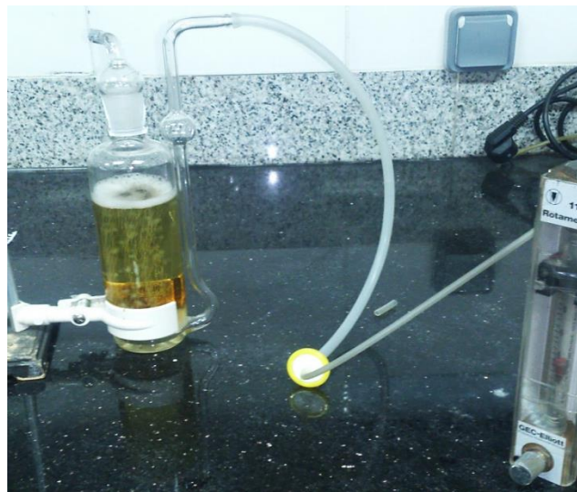
Figure 1. A 400-ml bioreactor, set at pH=5.1, T=28 °C and 1.4 vvm
