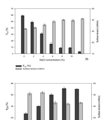
Surface Figure 3. Effect of the temperature (a), the osmolarity (b), and the pH (c) on the stability of the produced biosurfactant
