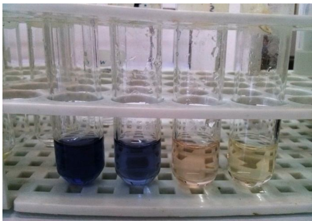
Figure 2. Reaction of different concentrations of starch with iodine reagent can generate various ranges of color.
