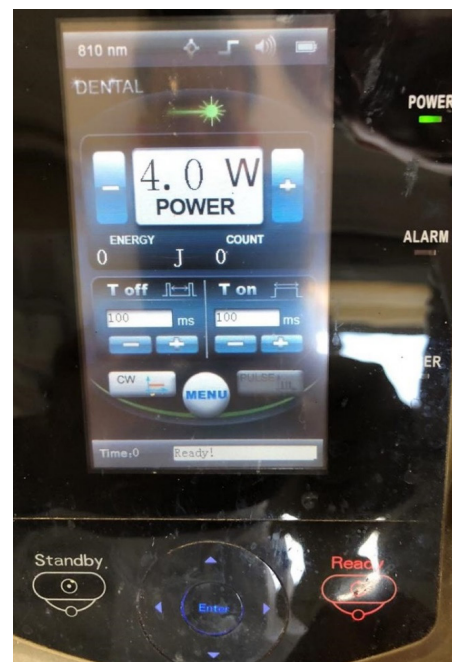
Figure 2. An 810 nm Diode Laser, With the Output Power of 4 W.(810 nm diode laser, Wuhan Gigaa Optronics Technology Co., Ltd.)
