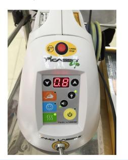
Figure 1. Picasso, AMD LASERS®, Wavelength 810 nm, Power 0.8 W.
