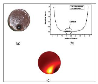
**Figure 2.** The Reconstructed image of an in-homogeneous phantom. The image of phantom (a) and the comparison between measured intensities around homogeneous and in-homogeneous phantom (b), and the position of defect can be seen in (c).
