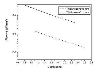
**Figure 1.** The penetration of laser light ( $\lambda = 780$  nm) for two different value of thickness of first layer.
