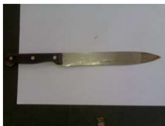
Fig. 6. The main part of the knife and the broken portion of the blade placed in apposition showing a perfect fit.
