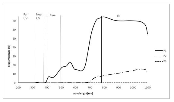
Figure 1. Spectral transmittance of the welding glasses tested in this study
