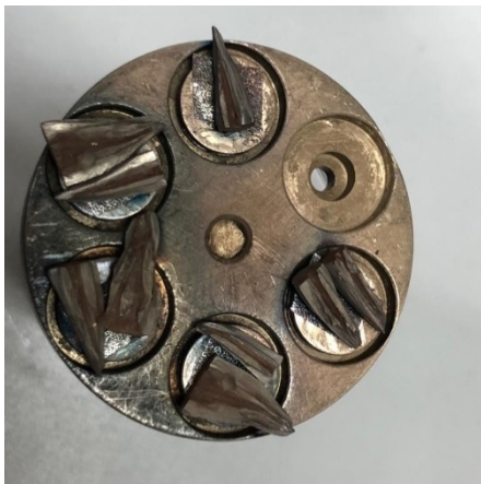
Figure 2. Covering of the samples with a layer of gold for SEM analysis was done
