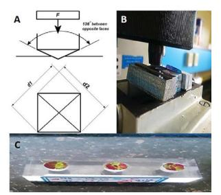
*Figure 1. A*) Schematic view of Vicker's microharness indenter. Two diagonals of the indentation left on the surface is measured and the microhardness is calculated; *B*) Microhardness testing machine. An indentation is made on the surface of specimen; *C*) Specimens in polycarbonate cylindrical mold shown after testing
