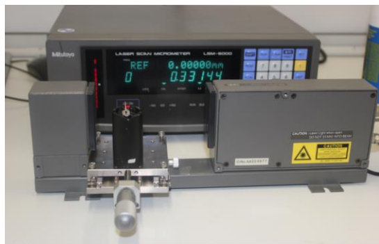
Figure 1: Travel crossed roller table connected to a micrometre perpendicular to the scanning laser beam of a laser scan micrometer (LSM 6000, Mitutoyo, Japan). D_0 level was established as a first reading achieved by LSM, where the specimens touched the laser beam; consequently, specimens were moved manually using micrometre ruler for further measurements
