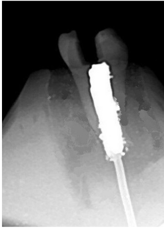
Figure 1. Radiographic confirmation of thermocouple in the pulp chamber
