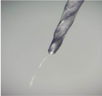
Figure 1. A stereomicroscopic view of wire slivering in F2 ProTaper file (20× magnification)
