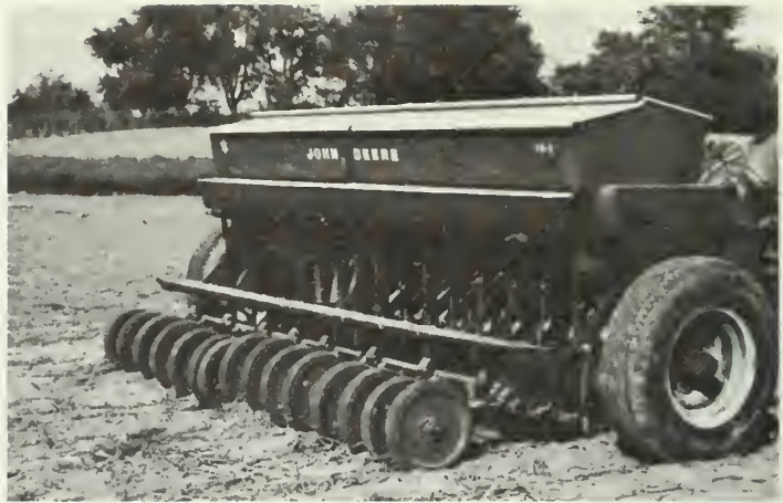
Small grain drill with band-seeding tubes, press wheels, and a grass-legume seed box. (Fig. 18)
