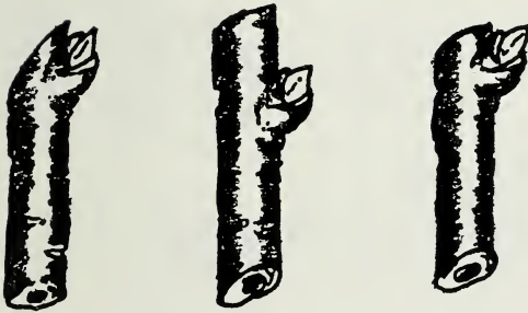
Cut at left has too sharp an angle; cut in center has too much stub left; and the correct cut is on the right. (Fig. 36)
