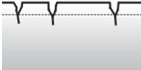
Figure 1.2 Sketch of pit corrosion and SCC initiation.
