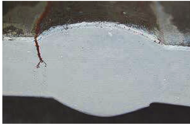
Figure 1.3 SCC between BM and HAZ
