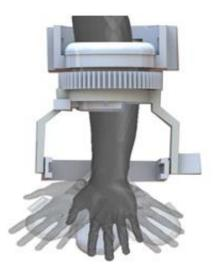
Fig. 12. Adduction and Abduction Movement of the Exoskeleton.
