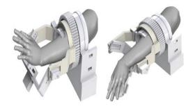
Fig. 10. Extension and Flexion Movement of the Exoskeleton.
