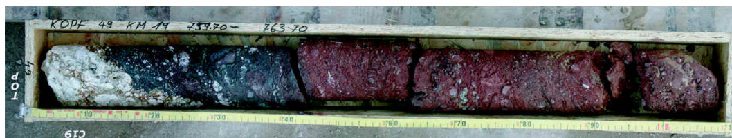
Fig. 1. : Box 49 containing the core at depth 759.70 m, characterized as “Aigion fault” core
