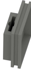
Figure 6.25: The 3D printed mount, to scale, used to hold both the RF calibration coil and the FLC100 fluxgate magnetometer. 10 turns of copper wire are wound around the mount, with a side length of 3.1 cm.
