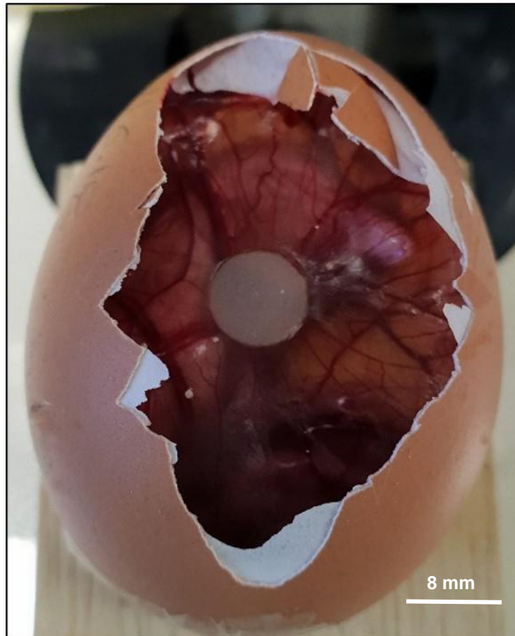
Figure 6.2 Whole disc of the experimental bone composite(0 wt % MCPM and 0 wt% PLS) photographed in ovo 7 days after CAM-grafting
